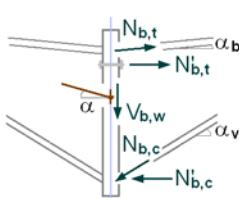
sign definition of statics: a positive axial force means tension, a positive bending moment produces tension at the bottom
