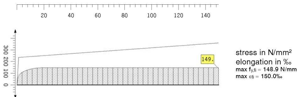
fire design at load level with the simple design method acc. to EC 3-1-2, 4.2
