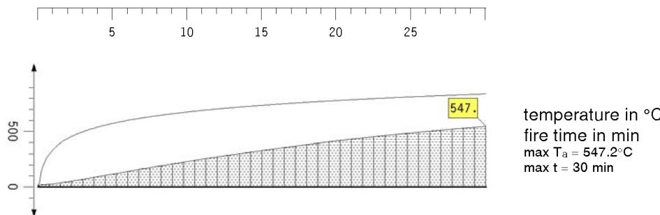
cross-section temperature acc. to t = 30.0 min: T<sub>a</sub> = 547.2 °C
