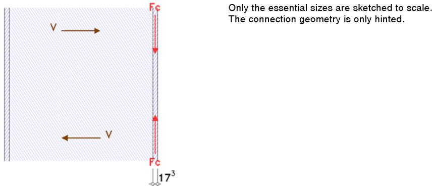
stress due to bending with shear force:  $V_{Ed} = 3.5 \text{ kN} \leq 492.5 \text{ kN} = V_{pl,Rd}/2 \Rightarrow \text{no effect}$
