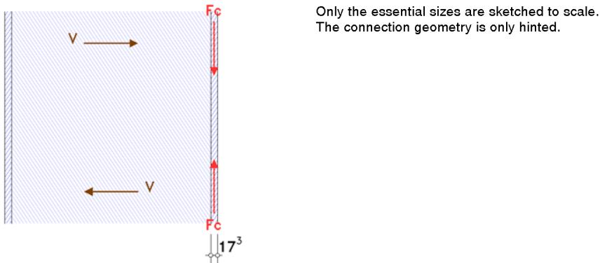
stress due to bending with shear force:  $V_{Ed} = 108.0 \text{ kN} \leq 492.5 \text{ kN} = V_{pl,Rd}/2 \Rightarrow$  no effect
