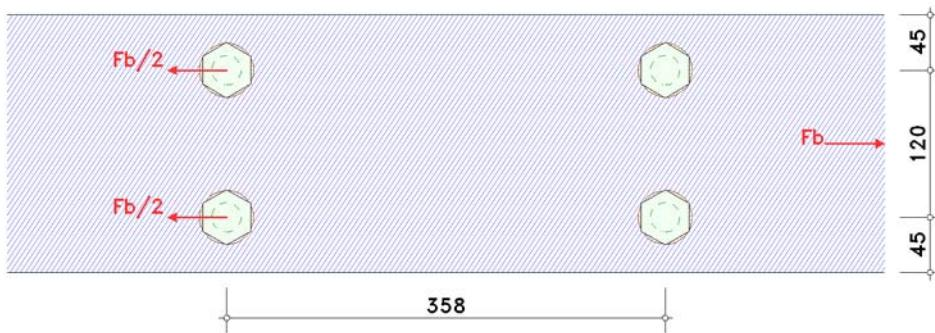
bearing resistance:  $F_{b,Rd} = (k_1 \cdot \alpha_b \cdot f_u \cdot d \cdot t) / \gamma_{M2} = 297.22 \text{ kN}$ ,  $k_1 = 2.50$ ,  $\alpha_b = 1.00$
