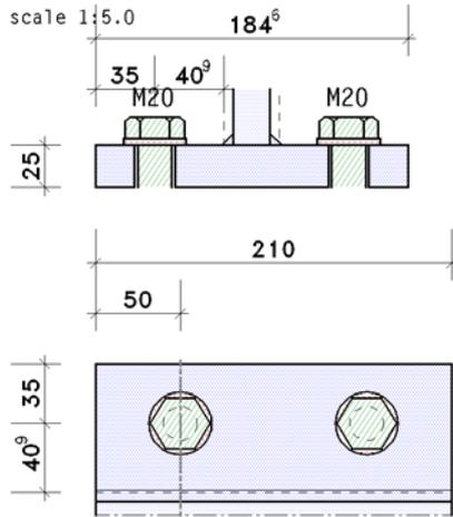
**T-stub flange** with thickness  $t = 25.0$  mm, length  $l = 184.6$  mm, width  $b = 210.0$  mm
