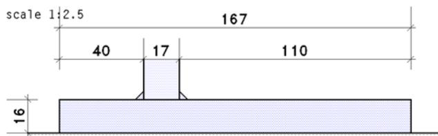
T-stub flange with thickness  $t = 16.0$  mm, width  $b = 250.0$  mm
