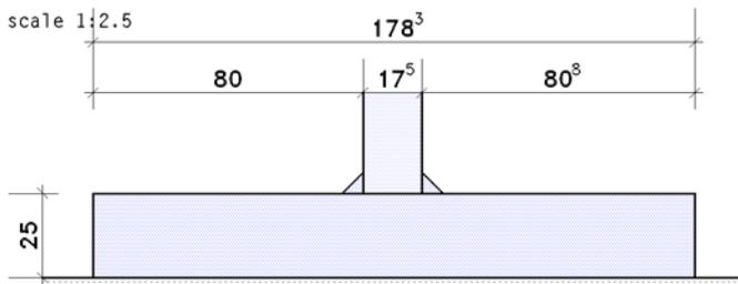
**T-stub flange** with thickness  $t = 25.0$  mm, width  $b = 340.0$  mm
