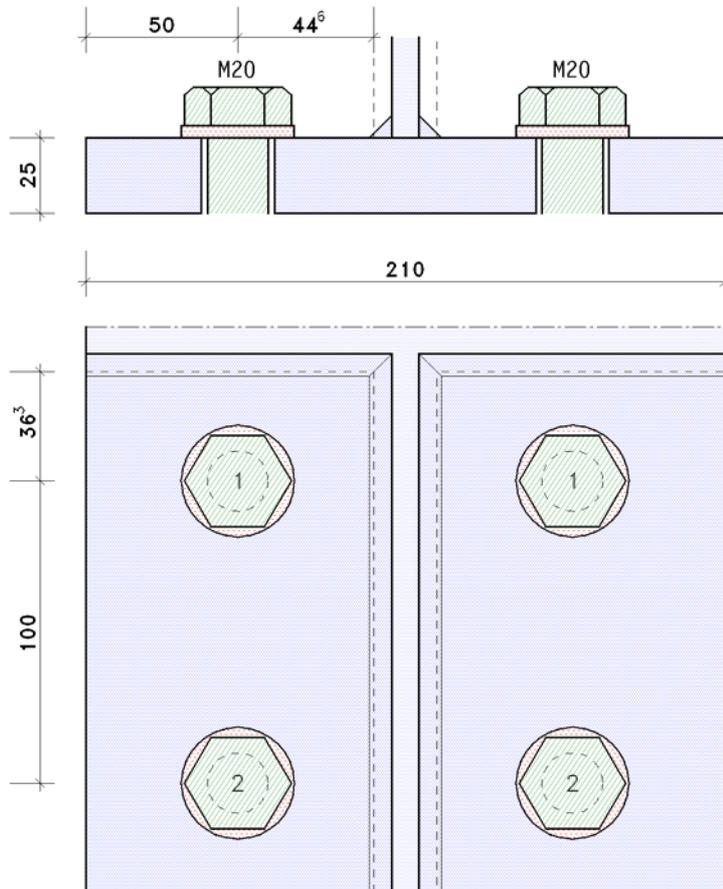
**T-stub flange** with thickness  $t = 25.0$  mm, width  $b = 210.0$  mm
