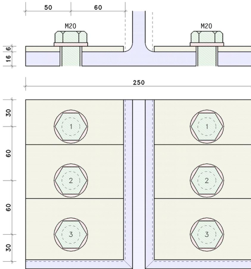
**T-stub flange** with thickness  $t = 16.0 \text{ mm}$ , width  $b = 250.0 \text{ mm}$
