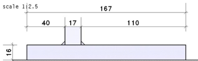
T-stub flange with thickness  $t = 16.0 \text{ mm}$ , width  $b = 250.0 \text{ mm}$
