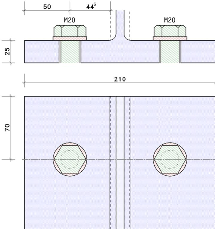
**T-stub flange** with thickness  $t = 25.0$  mm, width  $b = 210.0$  mm
