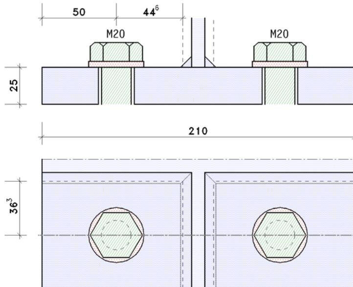
**T-stub flange** with thickness  $t = 25.0$  mm, width  $b = 210.0$  mm
