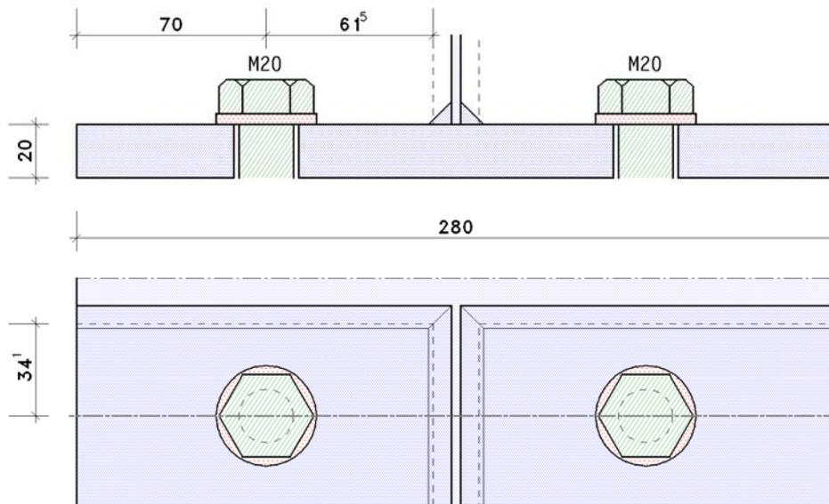
**T-stub flange** with thickness  $t = 20.0$  mm, width  $b = 280.0$  mm
