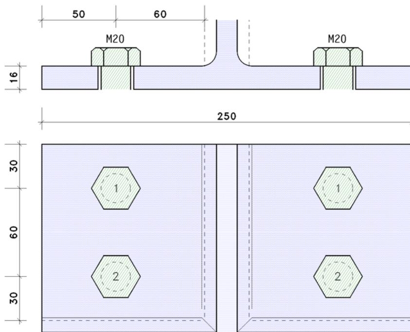
**T-stub flange** with thickness  $t = 16.0$  mm, width  $b = 250.0$  mm
