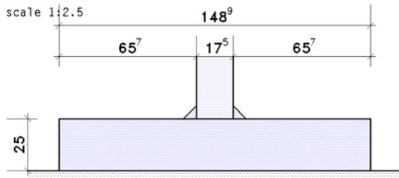
**T-stub flange** with thickness  $t = 25.0$  mm, width  $b = 280.0$  mm
