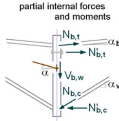
sign definition of EC3: a positive axial force means compression, a positive bending moment produces tension at the top
