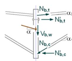
slope angle:  $\alpha_b = \alpha_v = \alpha = -7.40^\circ$
