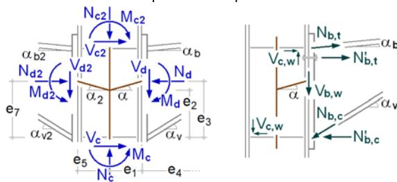
sign definition of EC3: a positive axial force means compression, a positive bending moment produces tension at the top
