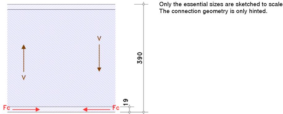
stress due to bending with shear force
