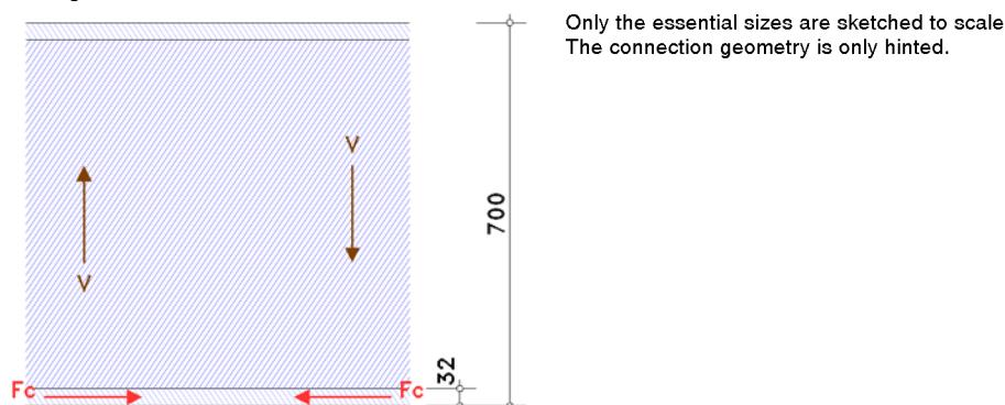
stress due to bending with shear force:  $V_{Ed} = 900.0 \text{ kN} \leq 930.1 \text{ kN} = V_{pl,Rd}/2 \Rightarrow$  no effect
