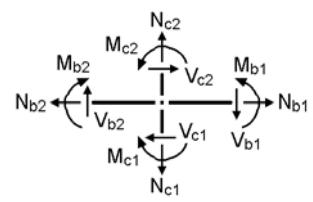
Lk 3:  $N_{j,b1,Ed} = 9.56 \text{ kN}$   $M_{j,b1,Ed} = -13.00 \text{ kNm}$   $V_{j,b1,Ed} = 17.93 \text{ kN}$  (right)
