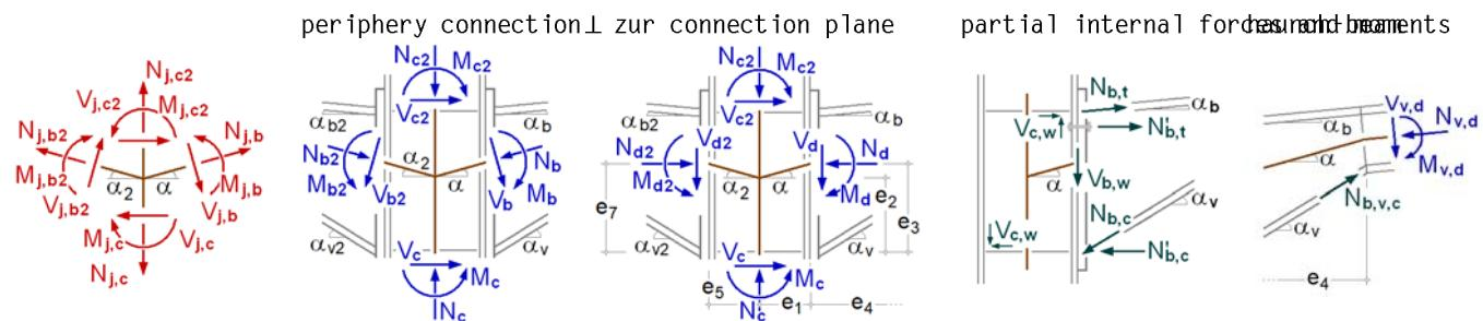
slope angle:  $\alpha_b = 0.00^\circ$ ,  $\alpha_v = 35.00^\circ \Rightarrow \alpha = (\alpha_b + \alpha_v)/2 = 17.50^\circ$ ,  $\Delta\alpha = \alpha - \alpha_b = 17.50^\circ$
