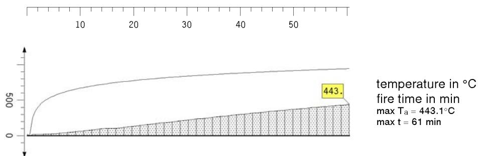
time saving due to moisture content of insulating material  $t_v = (p_p \cdot \rho_p \cdot d_p^2) / (5 \cdot \lambda_p) = 2.1 \text{ min}$
