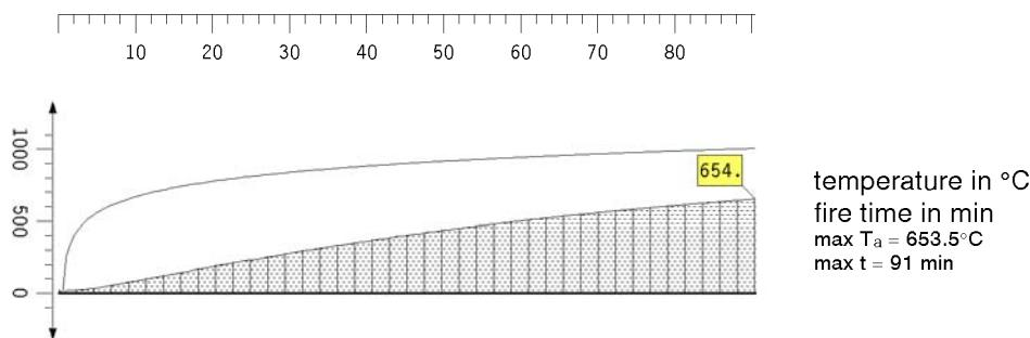
cross-section temperature acc. to  $t = 90 \text{ min}$ :  $T_a = 653.5^\circ\text{C}$
