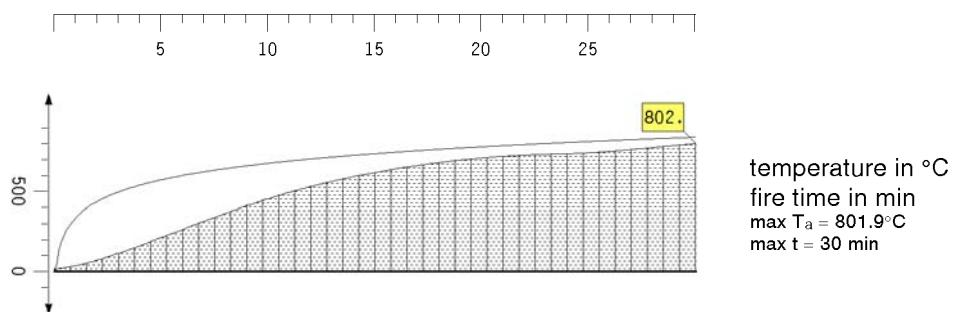
cross-section temperature acc. to  $t = 30 \text{ min}$ :  $T_a = 801.9^\circ\text{C}$
