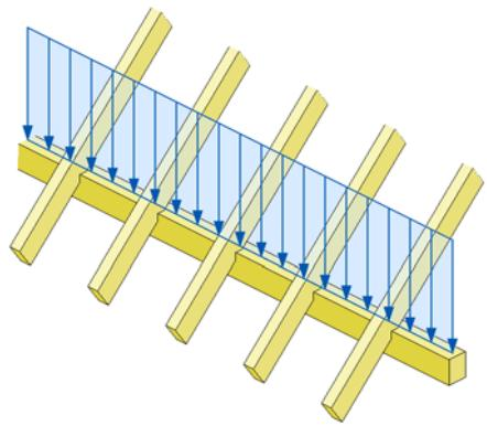
The values describe a line load in purlin running direction. Man loads that are to be applied only once per roof are not taken into account here.
