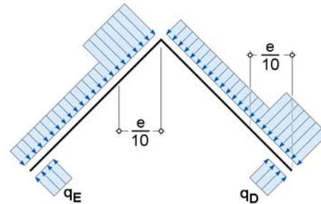
$q_D$  and  $q_E$  are acting only in the case of roof overhangs,
