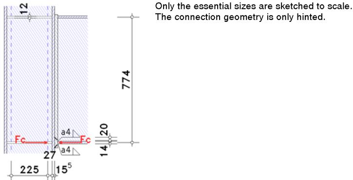
reinforcement of web with transverse stiffeners:
