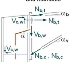
$$\text{angle of inclination: } \alpha_b = 2.0^\circ, \alpha_v = 14.6^\circ \Rightarrow \alpha = (\alpha_b + \alpha_v)/2 = 8.3^\circ$$
